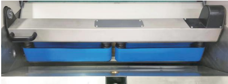
皮圈导棉出条结构 (标配) Apron guide cotton sliver structure (standard configuration)
